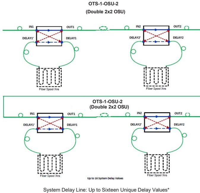
\*Various combination of delays based on each fiber spool delay values
